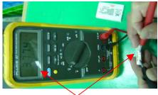
The nominal DC voltage in Lithium Battery is 3.7Vdc or higher. Above illustration show you the measurement of DC voltage in Lithium Battery is 3.774Vdc. Hence, this Battery is good.
