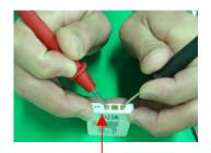
Measure the DC voltage of Lithium Battery as above illustration.
